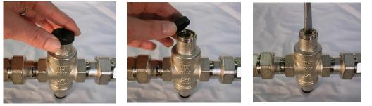
All Malgorani pressure reducers are tested before being packaged; during the test they are pre-set at the outlet pressure of 3 bars; the outlet pressure can be easily modified when the valve is installed on the water system.
